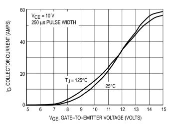
Figure 3. Transfer Characteristics
