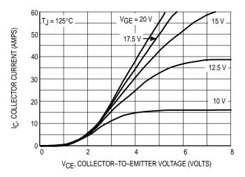
Figure 2. Output Characteristics
