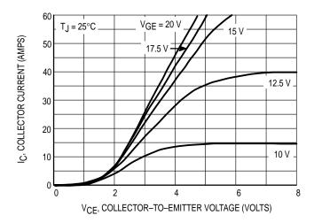
Figure 1. Output Characteristics
