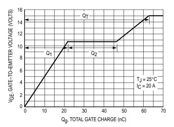
Figure 6. Gate-to-Emitter Voltage versus
