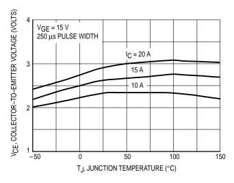
Figure 4. Collector-to-Emitter Saturation Voltage versus Junction Temperature
